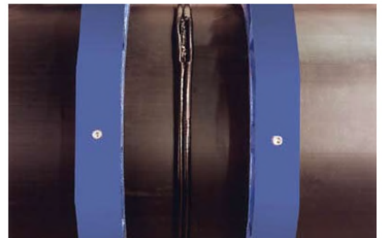
Fusion Pressure, Bead Roll Over & Cooling
