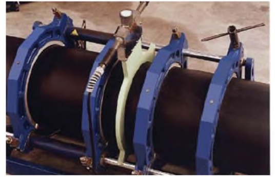
Heater Plate placed between pipe ends
